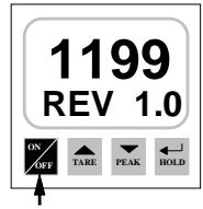
... and after 5 sec., the dynamometer starts to work with the auto - zero function and displays the applied weight.
