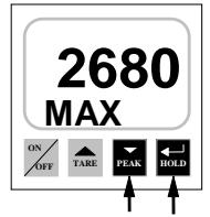
If the tare display is operating, pushing the button "PEAK", MAXT appears and, while the instrument goes on showing the tare, it will enter the peak weight.
