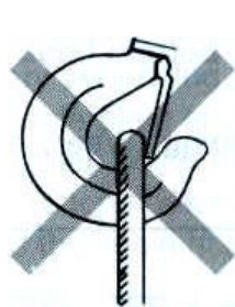
Incorrect handling example 1 (slinging tool hung on hook end)
