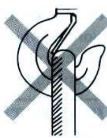
Incorrect handling example 3 (too thick slinging tool)
