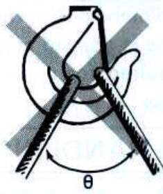
Incorrect handling example 2 (too wide slinging angle)
