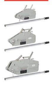
The REMA Gripper is a very robust wire rope hoist that can be used vertically, horizontally or at other angles, with a capacity of 800 kg, 1600 kg and 3200 kg. The shear pin and lever are reliable indicators for overloading.
