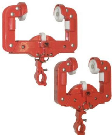
Elephant round cable trolleys are designed to relieve round power cables on cranes so that they do not hang down along the track. Cable sagging approx. 60 to 1000 mm.
